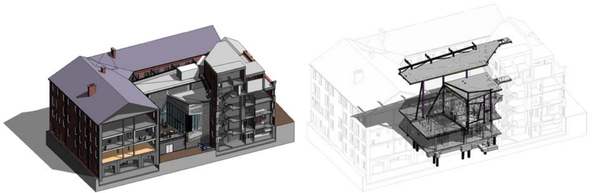
Architectural model with linked in structural model with regular data drops to maintain principal coordination throughout project
